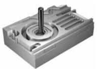
Shoulder, slot, pocket and face milling and more, this versatile cutter design allows a wide range of operations with the same tool. As a result of fewer tool changes you'll benefit from shorter cycle times as well as reduced tool inventory.
